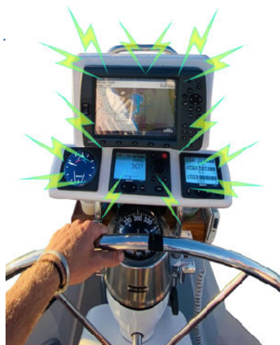
Ferrous metals and electronics will affect a nearby compass.
