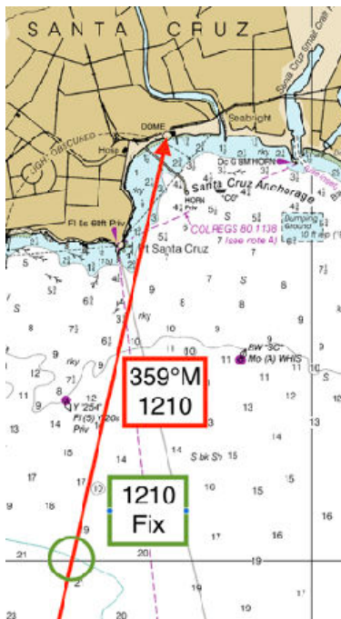
A fix using a bearing on the Casino dome at Santa Cruz, California, and the chart's 20 fathom depth contour.
